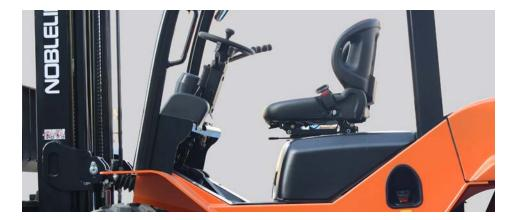
The large, ergonomic cab and user-friendly design with cushioned rubber floor mat, ensures operator comfort throughout the entire work shift. Low entrance height provides operator easy and safe access. Deluxe suspension, fully adjustable seat reduces vibration to the driver to effectively reduce driver fatigue for all sizes of operators.
