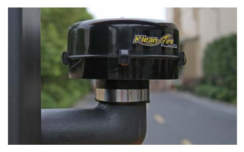
Centrifugal pre-cleaner removes 90% of impurities, rain, debris, dust and dirt from intake air before the air reaches the filter element. This reduces engine wear, minimizes downtime and improves fuel economy.
