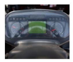
Large LED display and CAN Bus function provides truck status information: parking brake, driving direction, speed, hour meter and fault codes.
