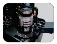
Powerful AC drive motor from Schuabmuller is paired with High Capacity ZF gearbox and Intorq electro magnetic brake provides speeds up to 5 MPH. The use of quality drive wheel from German manufacturers Rader Vogel or Wicke helps to ensure the life time of Pu tyre.
